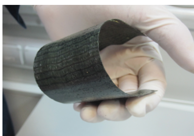
Fig.1. Photograph of a sample of flexible composite based on modified carbon fiber.
