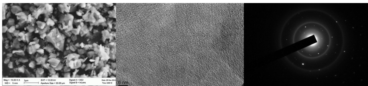
Fig.1. Common view (SEM, left), high resolution TEM image (middle) and the electron diffraction pattern (right) of shungite.
